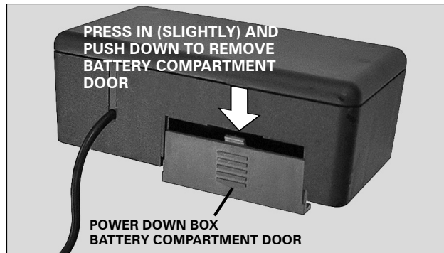
FIGURE 2: Power down box battery compartment door removal.
